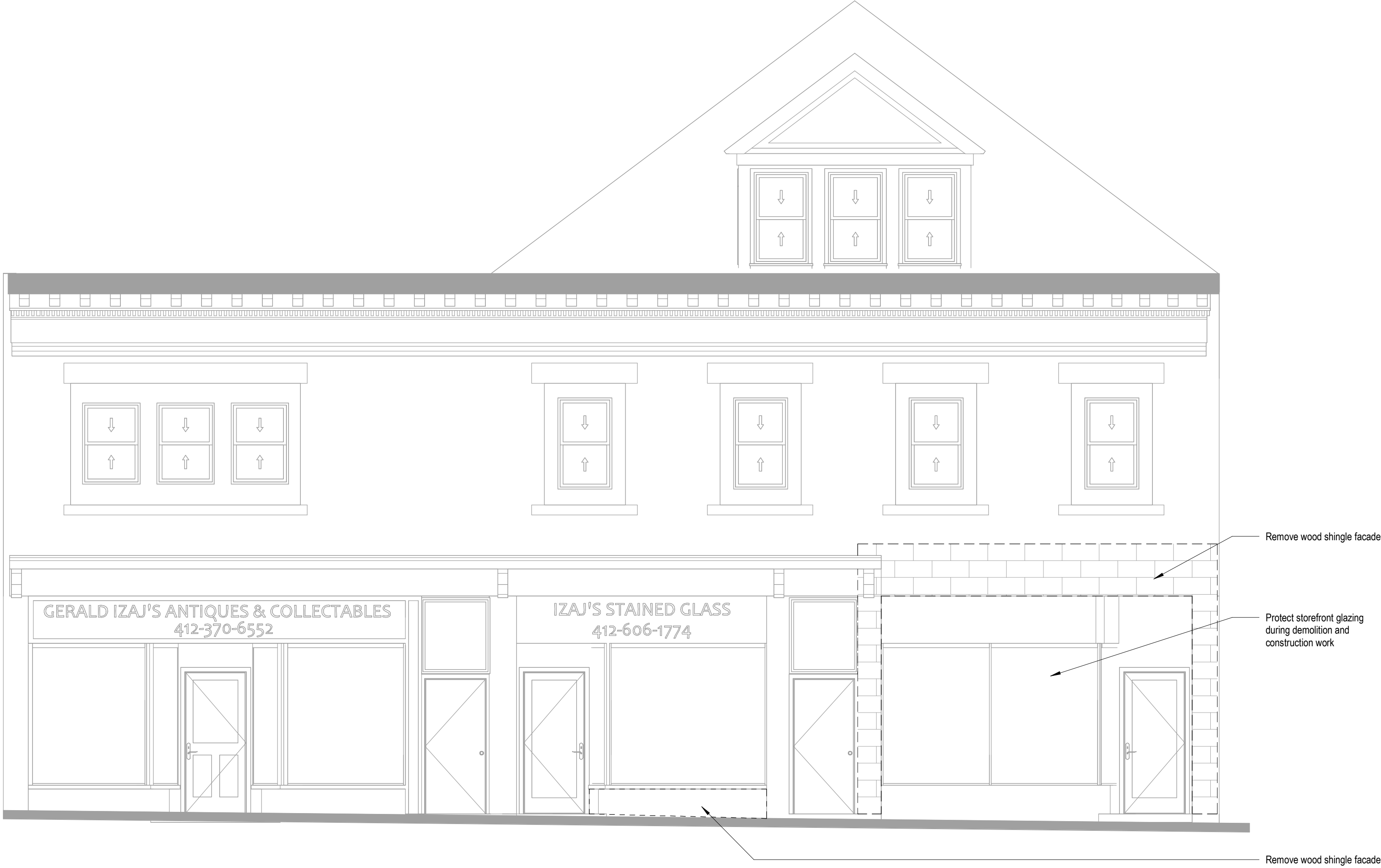
1 Front Building Elevation - Demolition 1/4" = 1'-0"
